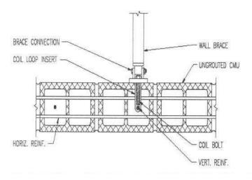
Straight coil loop insert attached to rebar with perpendicular rebar between it and face shell to receive brace.
