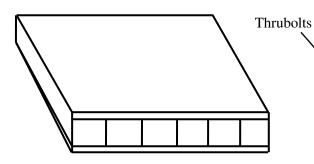
4X4 or 4X6 with plywood top and bottom to stiffen enough to span soft spots
