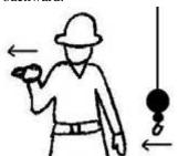
**TROLLEY TRAVEL** – With palm up, fingers closed and thumb pointing in direction of motion, hand is jerked horizontally in direction trolley is to travel.
