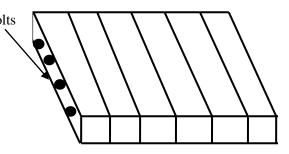
4X4 or 4X6 with thrubolts to stiffen enough to span soft spots
