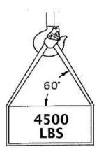
Actual Sling Capacity = factor X rated capacity
